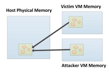
3. If the attacker VM's physical memory is chosen to back both pages (refer to our USENIX paper to see how this can be done), the attacker can then trigger Rowhammer to modify the memory of the victim. As shown in the figure below, DRAM is organized in rows, and repeated activation of two rows (e.g., row i-1 and i+1) can trigger a flip in another row (e.g., row i).
